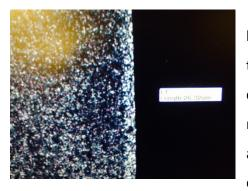
This allows for performance that has not previously been seen from lightweight alloys and gives them the ability to be used in applications that have been reserved for steel components due to its wear resistance. When tested in mixed regime sliding, ArmorTi<sup>®</sup> applied to a Ti-6-4 substrate exhibits a wear rate of 5.0 x 10<sup>-6</sup> mm<sup>3</sup> / J, while untreated specimens exhibit a wear rate of 1.0 x 10<sup>-3</sup> mm<sup>3</sup>/J.
